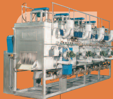
Gas belt furnace 600°C
