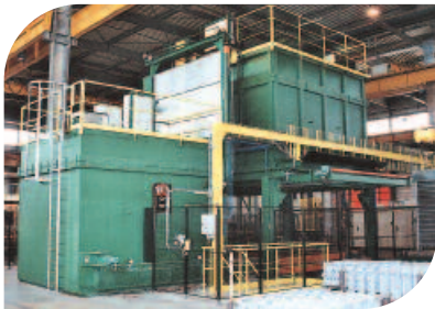
Quenching furnace 550°C, total load submersion, with tempering furnace
